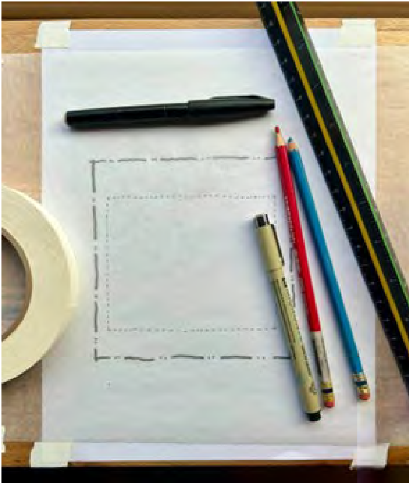
A few basic tools and techniques is all it takes to begin a conceptual site plan. Shown is a 100-foot x 100-foot, 10,000 square foot lot with setbacks at 1:20 scale, where 1 inch equals 20 feet.
